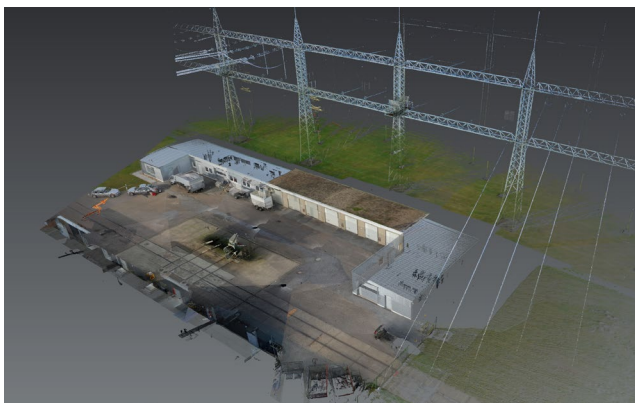
3D point cloud: as-built documentation electric switchgear
