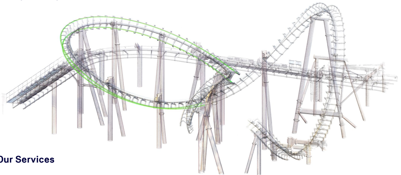
3D point cloud: as-built documentation of a rollercoaster
