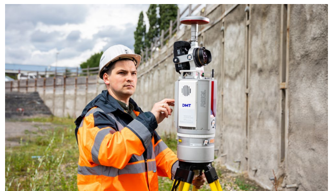
Scanning an excavation pit: determining volume and condition
